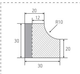
\* In the case of installing 12mm-thick cladding or flooring, the baseboard pieces can be cut to 30 x 30mm to fit them to the required dimensions.
